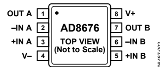
Figure 2. 8-Lead MSOP (RM-8)
