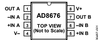
Figure 1. 8-Lead SOIC_N (R-8)
